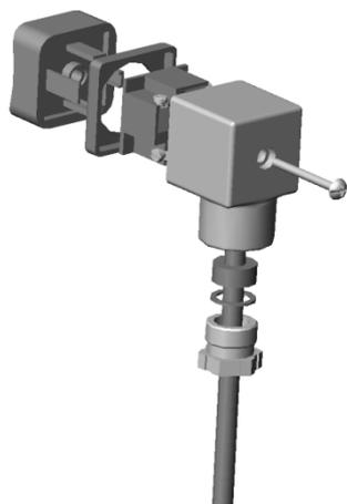
Figure 1 – Exploded view of the connector
